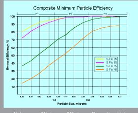
Values are Minimum Efficiency Reporting Values (MERVs) when evaluated per ASHRAE Standard 52.2. The Camfil S-Flo incorporates an exclusive blend of synthetic micro fibers that are electrostatically enhanced during the fiber manufacturing process to enhance particle capture efficiency. Biologically inert, these fibers will not support microbial growth. The media is color-coded to allow quick identification of filter efficiency.
